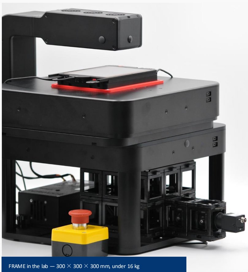
Optical cubes, pre-aligned off the instrument
